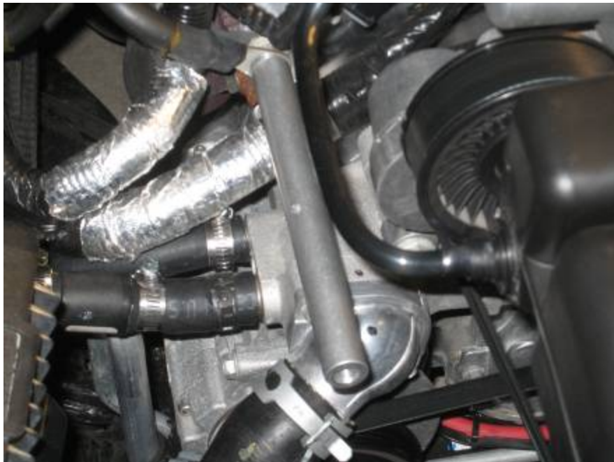
Figure 2: Aluminum Rod Secured to Engine Block
