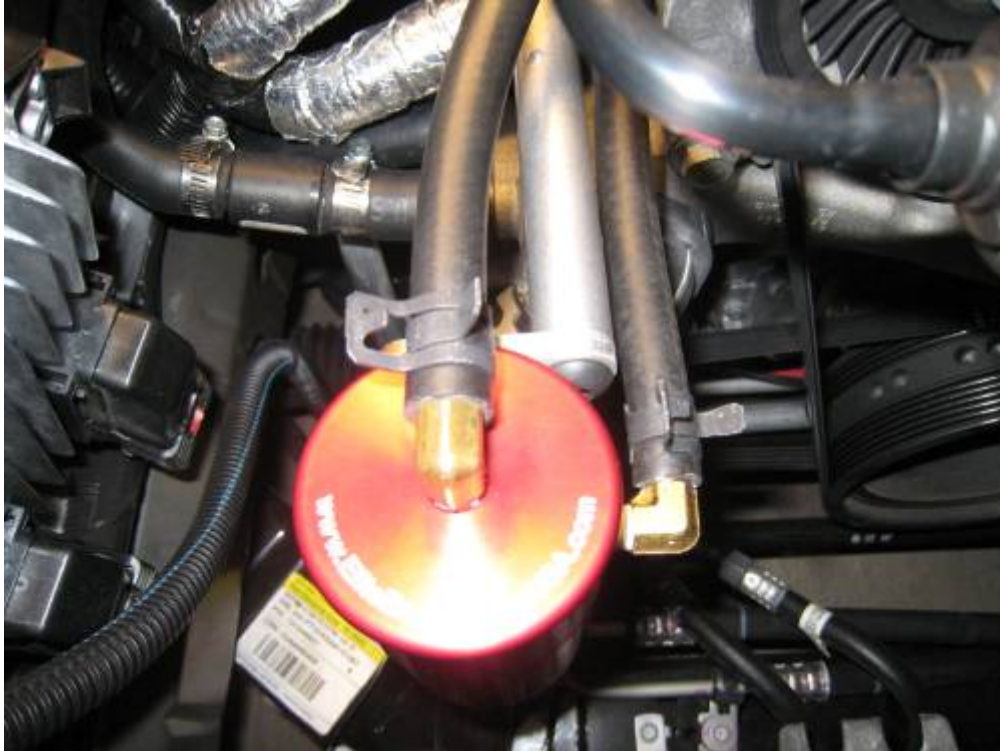
Figure 9: Hoses Installed on Catch Can
