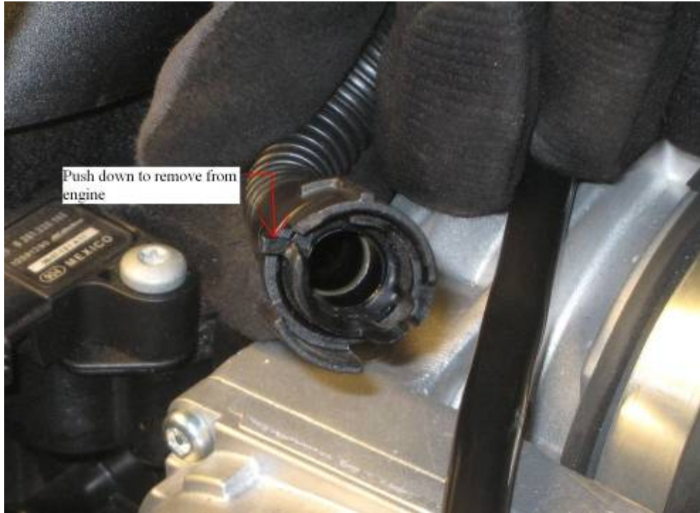
Figure 5: Removal of Stock PCV Line
