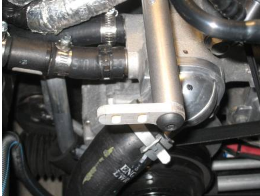
Figure 3: Bracket Installed on End of Rod
