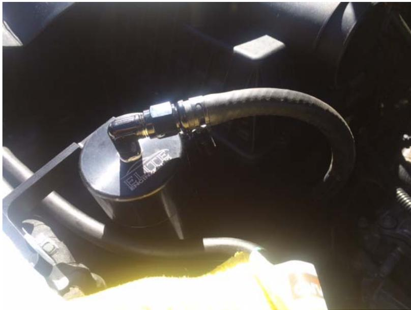
Take the end of the Intake Manifold side for the PCV and attach the supplied hose and clamp to it. We routed it this way because we found that the PCV couldn't pop back out easily.
