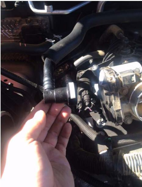
Follow this hose all the way back to near the driver side firewall. There will be another hose clamp on that end. Grab your needle nose pliers, take the clamp off, and pull the hose off.
