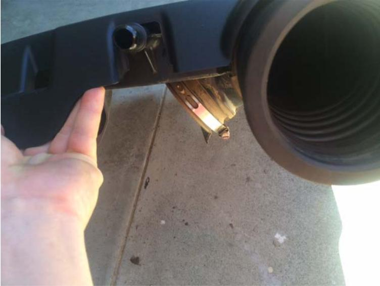
Push down on the gray part of this connector. Rotate till the end that is currently pointing towards the firewall, towards the hood. Pull towards the passenger side of the car and the end should come right off. After this you can remove the oil cap. Then pull the whole engine cover towards the front of the car. It should come off.
