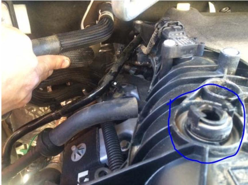
You have now removed the PCV hose from the engine. Cut each end off but make sure to leave enough room to attach the Rubber hose that was included with your kit along with the hose clamp shown below. We recommend you put some lubricant before trying to push any hose ends on. A little goes a long way!
