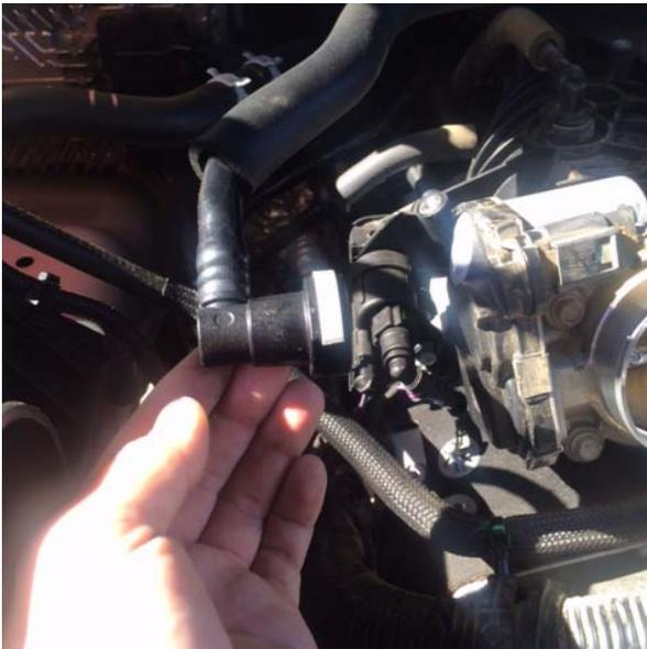
We assembled and mounted the catch can on the passenger side of the vehicle using a bolt to the left of the radiator. The bolt is pointing towards the firewall. Don't forget to put some Teflon paste or Teflon tape on the ends of the threads going into the can since they are NPT threads. The AN sides will not need any Teflon paste or Teflon tape.
