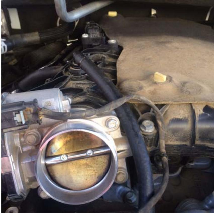
After routing this hose, attach the hose ends. We can go now ahead and attach it to the side port (outlet port) of the Elite Engineering Catch Can.
