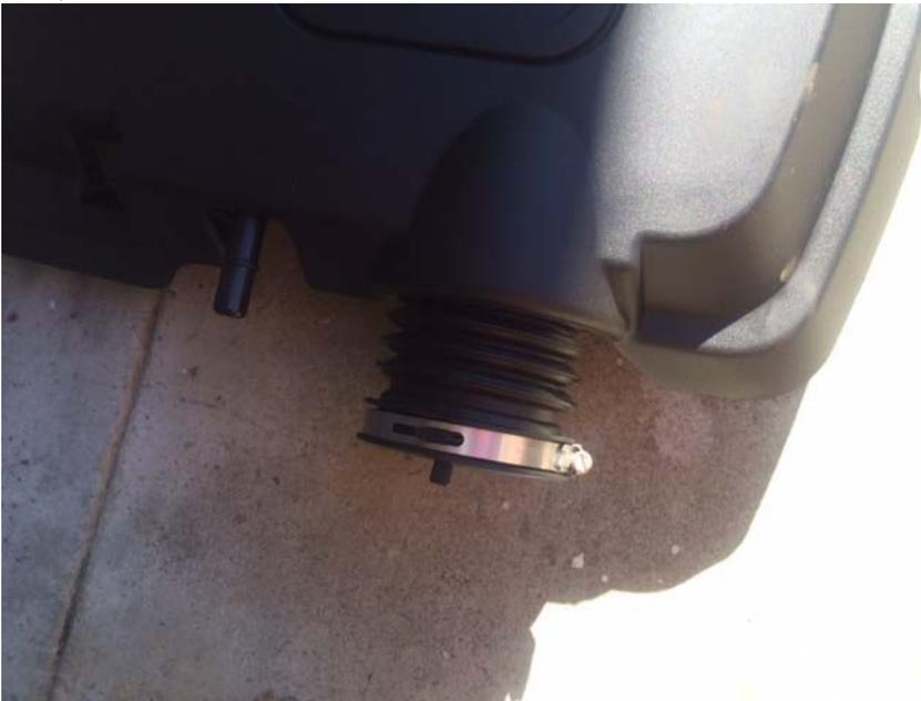
Loosen the throttle body hose clamp. Picture of location is below. We found it was easiest if you go to the passenger side of the car and do it. (Took the picture off the car for better illustration)
