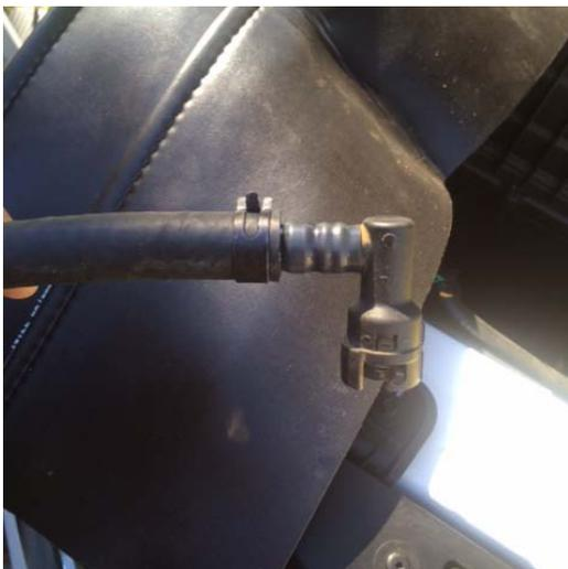
Stick the PCV for the Valve Cover end back on. You should hear a click. Then run the rubber line keeping clear of the exhaust manifold and pulleys to the catch can.
