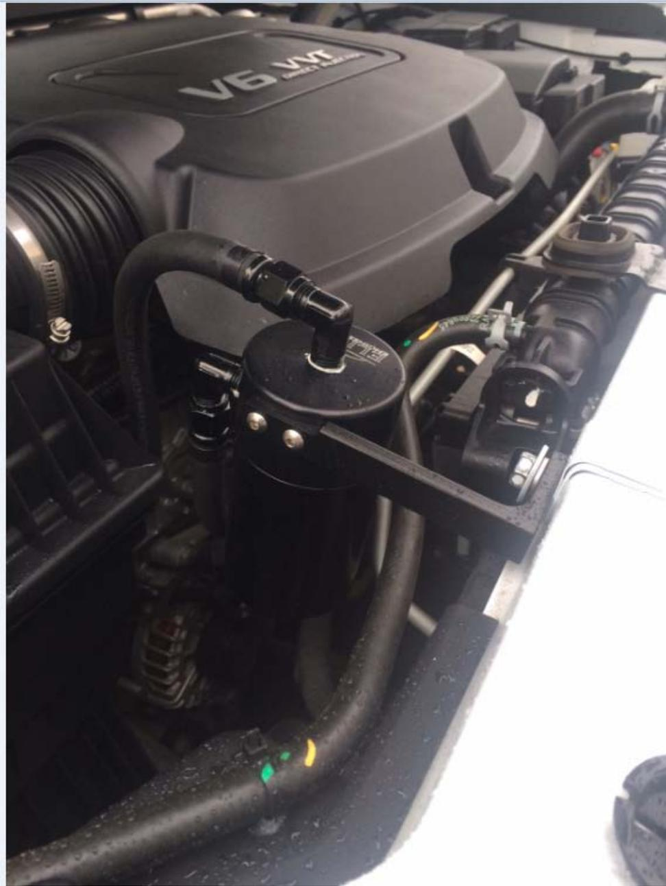
One end of the PCV hose goes to the passenger side valve cover while the other side is located in the intake manifold. To remove the end on the valve cover, feel around the back of the fitting. There will be a nub that sticks out. Push that towards the driverside and then lift up. It should come right off.
