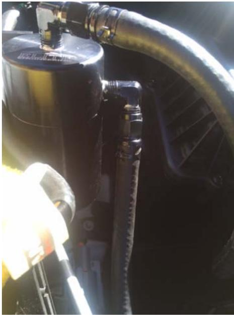
The install of the Elite Engineering Catch Can is complete! From now on, no oil should enter into the intake manifold through the PCV.
