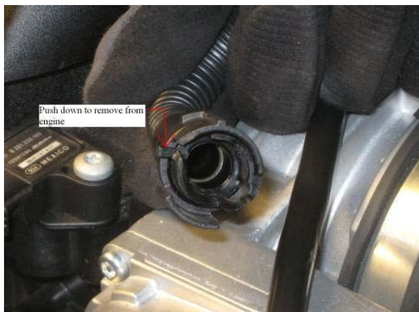
Figure 5: Removal of Stock PCV Line
