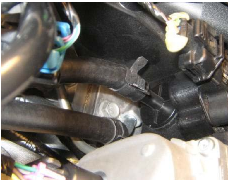
Figure 6: Rubber Hoses Installed on PCV Outlet and Inlet
