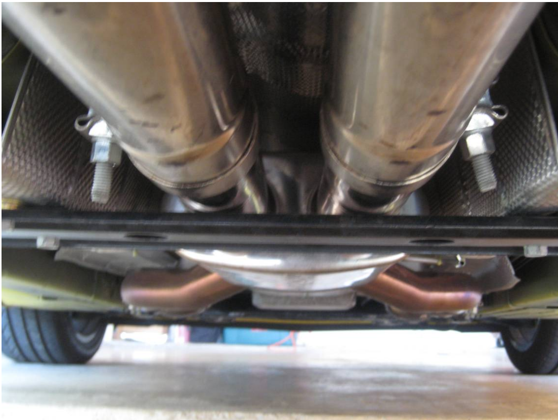
Picture of Stock Tunnel Brace
