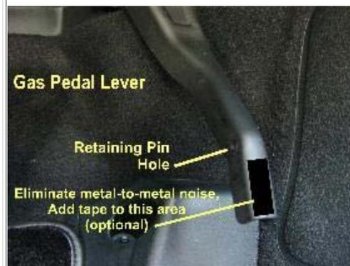
This is how the backside of your stock pedal looks with the tension spring. The retaining pin has been removed from this picture.
