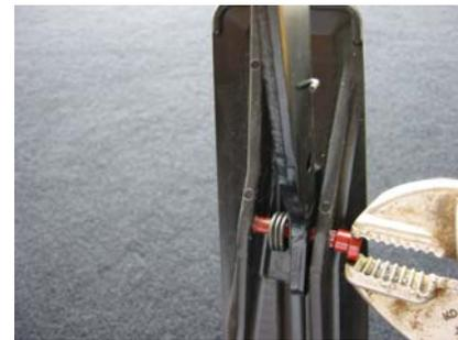
Some members have found this tool to be very useful when trying to remove the retaining pin >>>
