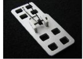
Next, insert the "supplied" 3/16" shoulder bolt into the Gas Pedal and begin to push it through the Gas Pedal Lever. Once the shoulder bolt has been started, install the Tension Spring Arm.
