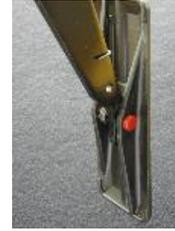
With a pair of Vise-grips, reach around your stock gas pedal and remove the retaining pin. It's a press fit so you may need pull with some force to remove it. In some cases you may need to pry it out with a screwdriver or sharp wood chisel.
