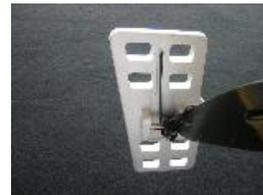
Once the spring is in the correct orientation, using the 3/32" Allen wrench and tighten the shoulder bolt.
