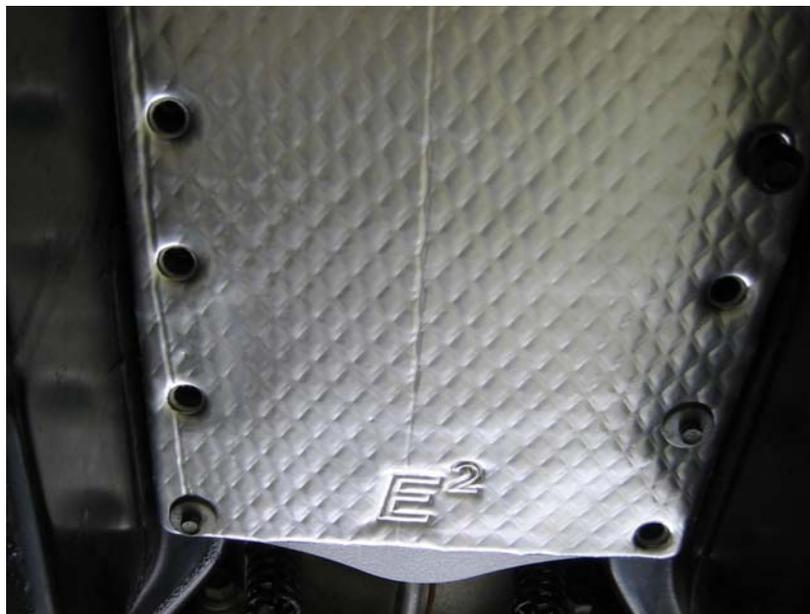
Start the rest of the screws and then carefully **hand-tighten** them using the 6-inch extension with the 8-mm socket. Snug them all down sequentially until they are completely seated.
