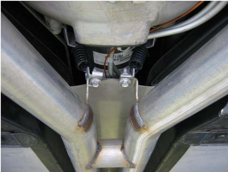
Below is a shot of the stock H-pipe and center exhaust section removed. At the very top bottom of the picture, you can also see the flanges of the exhaust manifolds. Remember, the exhaust manifolds do not need to be removed for the installation of Elite's Tunnel Plate. You can also see the location of the O2 sensors and mounting brackets.
