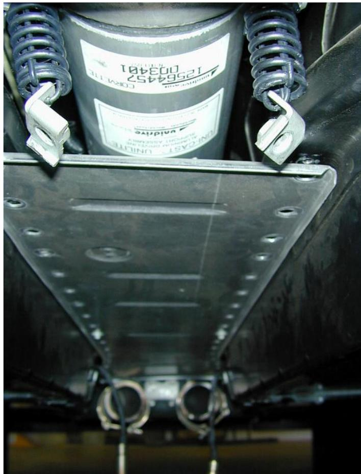
This is essentially what your tunnel should now look like. A great opportunity to inspect the torque tube and central tunnel area and to clean up a bit while it's exposed. Note: The blue thermocouple wires in the pictures are left over from our Tunnel Plate Temperature Testing.
