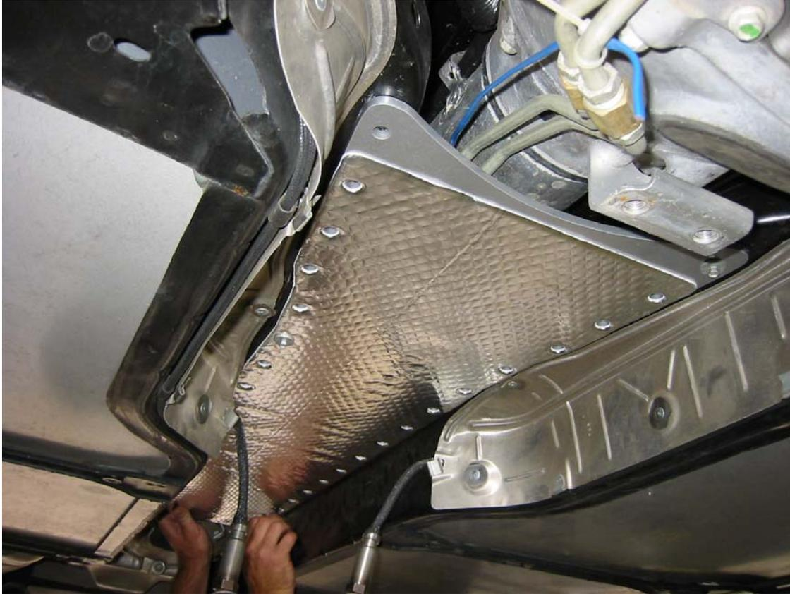
You should be able to read the **E<sup>2</sup>** logo from underneath and it should be at the rear of the tunnel. Carefully lift it into place and start two of the screws on opposite sides near the center of the plate to hold it in position and to bear its weight. You **WILL** reuse the original (36) screws that we removed during the first section. Even with the 3/8" thick plate, there is plenty of thread left in the original screws.
