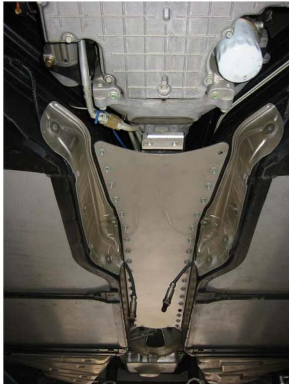
The stock plate is held in place by (36) 6x1.25 mm bolts. To remove the stock plate, use an 8 mm socket on a 6-inch extension to first loosen, but not remove, two of the center-most screws, one on each side opposite each other. Then completely remove the other 34 screws. See the picture below. Finally, remove the two you first loosened while supporting the plate to prevent it from falling. Then carefully move the plate away from the car.
